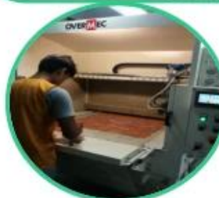
Glue Machine for Leather
