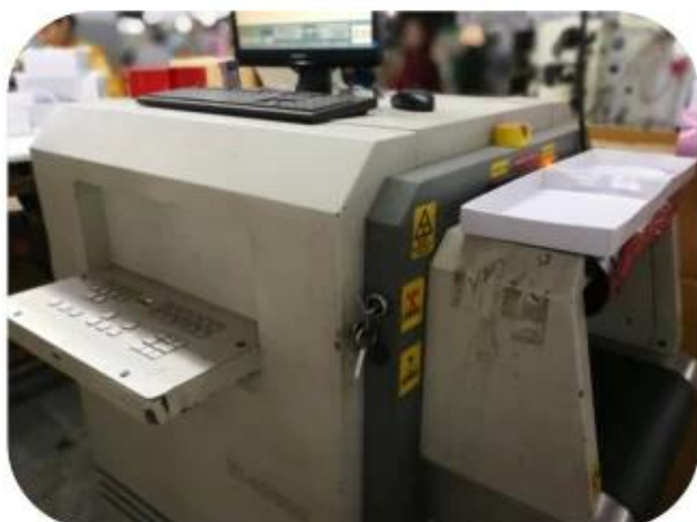
11.1 Finished Products Metal X-ray Detector
