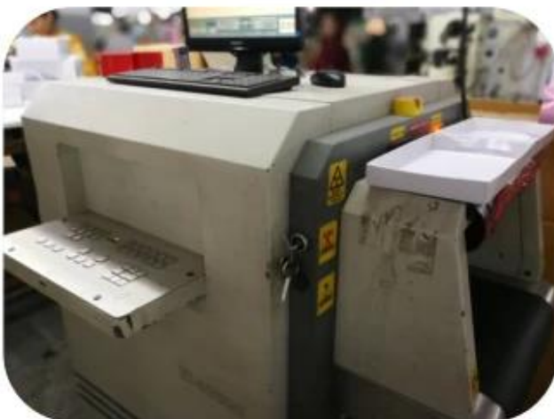
11.1 Finished Products Metal X-ray Detector
