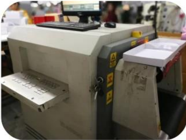
11.1 Finished Products Metal X-ray Detector
