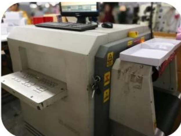
11.1 Finished Products Metal X-ray Detector
