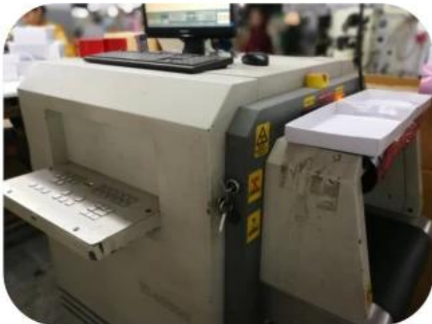
11.1 Finished Products Metal X-ray Detector
