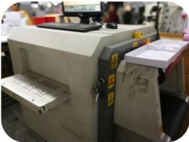
11.1 Finished Products Metal X-ray Detector
