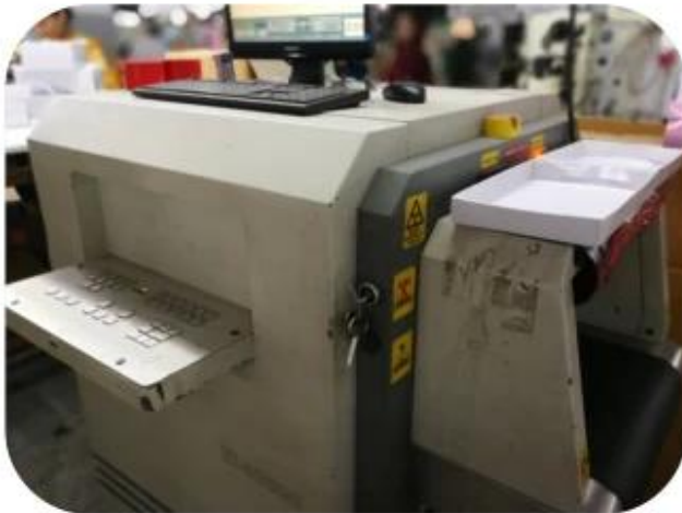
11.1 Finished Products Metal X-ray Detector
