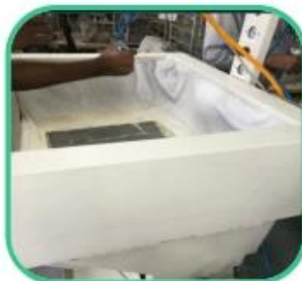
Glue Machine for Lining
