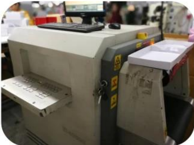
11.1 Finished Products Metal X-ray Detector
