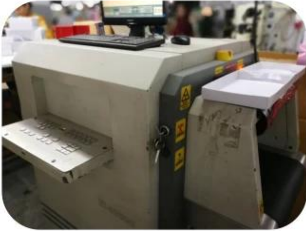
11.1 Finished Products Metal X-ray Detector
