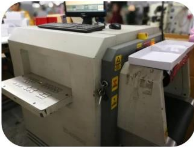
11.1 Finished Products Metal X-ray Detector
