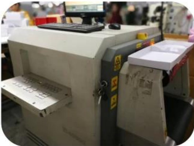
11.1 Finished Products Metal X-ray Detector
