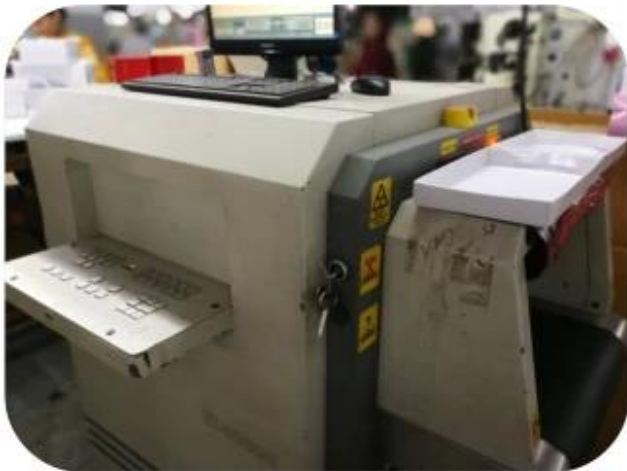
11.1 Finished Products Metal X-ray Detector
