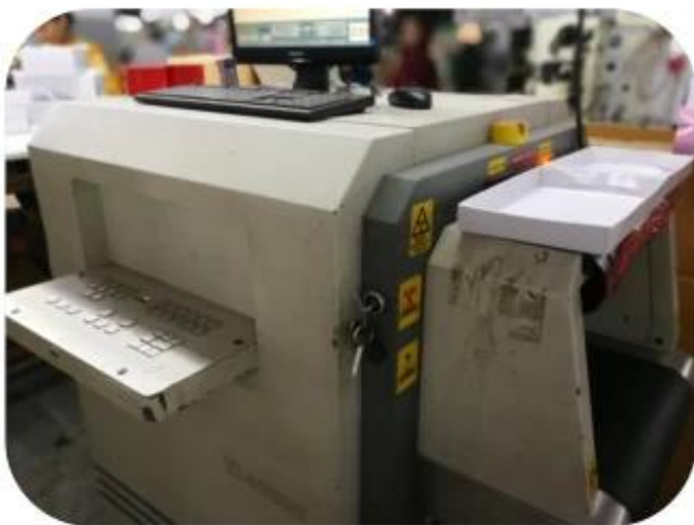
11.1 Finished Products Metal X-ray Detector
