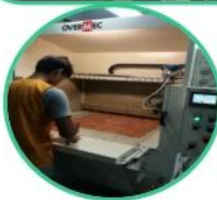
Glue Machine for Leather
