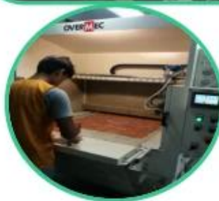
Glue Machine for Leather
