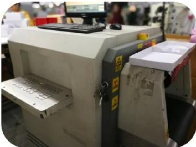
11.1 Finished Products Metal X-ray Detector
