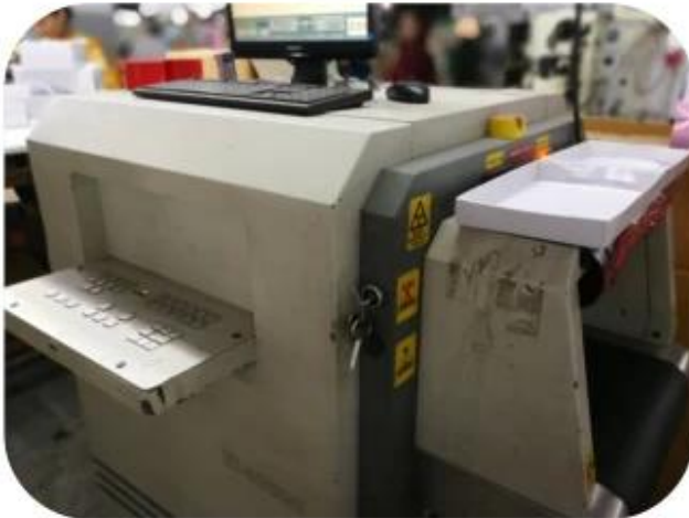
11.1 Finished Products Metal X-ray Detector
