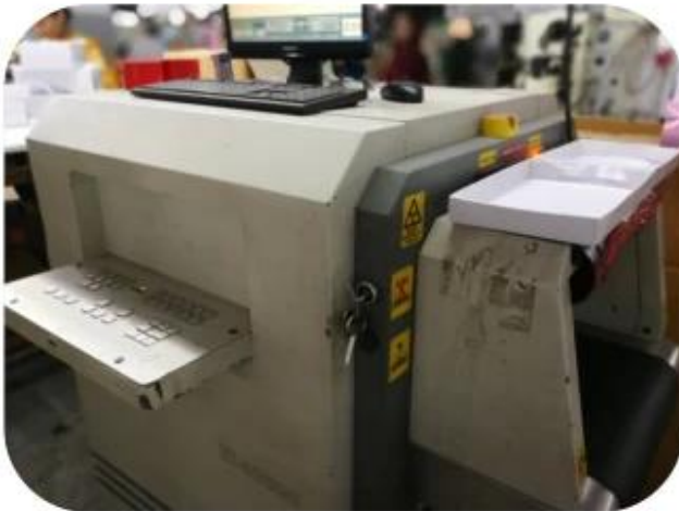
11.1 Finished Products Metal X-ray Detector
