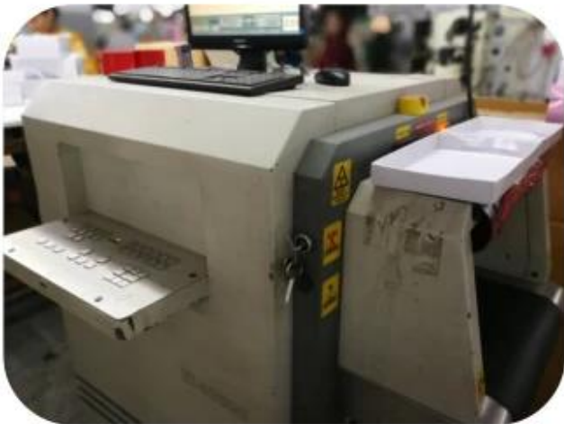
11.1 Finished Products Metal X-ray Detector
